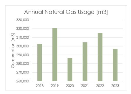
Natural gas usages have seen a lot more variability due to overall winter temperature changes and HVAC equipment reaching the end of life and needed to be replaced. For example, a new boiler was installed in October 2023 which has resulted in 1.64% reduction in weather normalized (considering the impacts of a warmer/colder winter) natural gas usage in the past 2023/24 winter. The benefits of this project are expected to continue over the useful life of the boiler.
